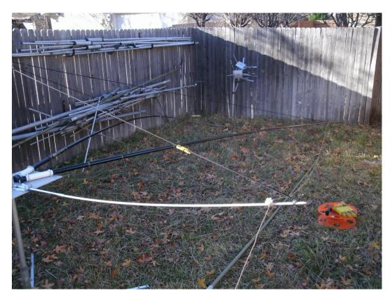
No amount of adjustments could keep the tips of the antenna up in the air. It appeared that the weight of the wire was just too much for the poles. The poles still may be a good idea, but I would likely have to use lighter wire or a smaller antenna system.
