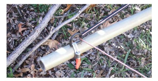
I used the same method to attach the D-rings to the end of the support tubes.
