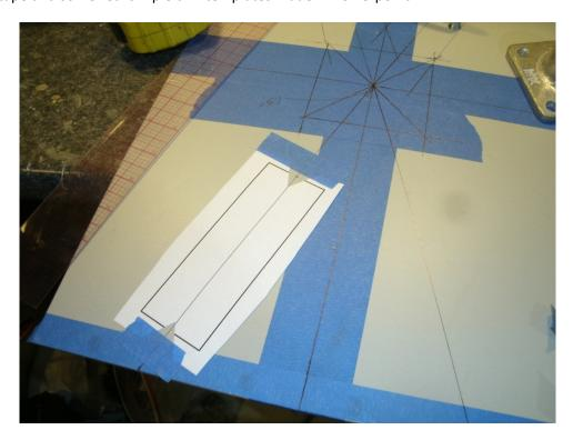
The white template is used to mark the holes for the U-bolts to hold down the spreaders. In looking at the spreaders, I decided that I wanted to reinforce the area that the U-bolts would clamp on. As it turns out, common 1" PVC water pipe worked just fine. I simply glued a 6" section to each spreader.
