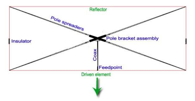
The first thing I had to calculate is the approximate length of the spreaders. I used P**ythagorean** theorem. That is  $a^2 + b^2 = c^2$ . This is one of those very common equations that can be used with right triangles. So, here we go:
