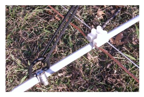
I went ahead and installed a center support rod on the other side of the center plate to hold up the reflector center wire a little better.
