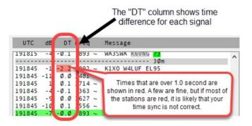
If you are operating in the field (for more than a day or two) or at a location with no Internet access, I suggest using a USB GPS Dongle to synchronize your computer's clock.
